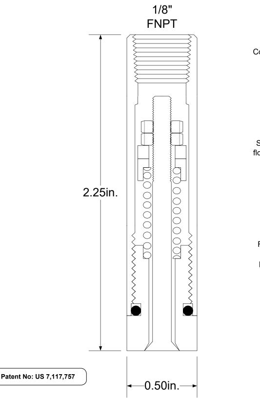
Housing and All Components other than spring are 316 Stainless Steel.
